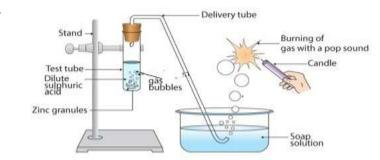
What happens when dilute sulphuric acid is replaced with concentrated solution of sodium hydroxide and heated in the experiment shown in the above diagram?
