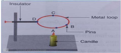
The circular metal loop is heated at the point A with the help of a candle flame. As per above data answer the following
